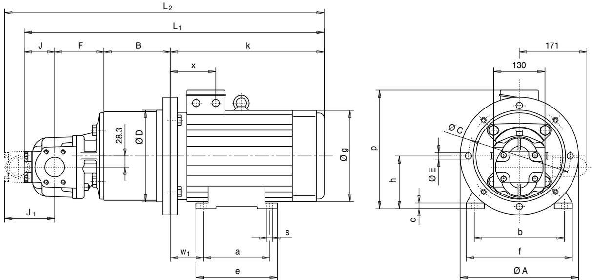
Motorbauform: IM B35 (IM V15; IM V36)
