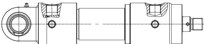
01 – Pivot lug with joint bearing
