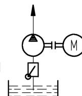
When operating a pump that has to pump via a non-return valve into a pressurized circuit (e.g. reserve pump in a lubricant circuit), intake difficulties can occur if the suction line is filled with air. In this case the pressure line must be vented directly upstream of the non-return valve. If a venting nozzle is not inserted, the volume of the pressure line between the pump and non-return valve must be at least 75% of the suction line volume.
