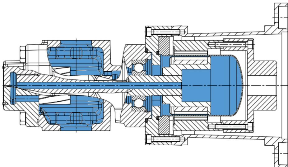
Versions with magnetic coupling are used when absolute leak-proofness is required on the shaft seal or when being operated with supply pressure on the suction side. The magnetic coupling is leak-proof within the permissible technical limits.
