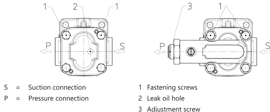
To change the direction of rotation of the gear pump, turn the end cover or the pressure relief valve 180°.
