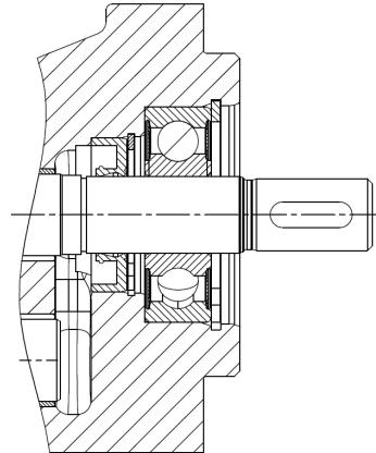
Rotary shaft seal with roller bearings
