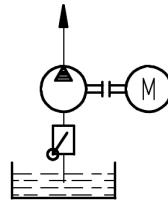
When operating a pump that has to pump via a non-return valve into a pressurized circuit (e.g. reserve pump in a lubricant circuit), intake difficulties can occur if the suction line is filled with air. In this case the pressure line must be vented directly upstream of the non-return valve. If a venting nozzle is not inserted, the volume of the pressure line between the pump and non-return valve must be at least 75% of the suction line volume.
