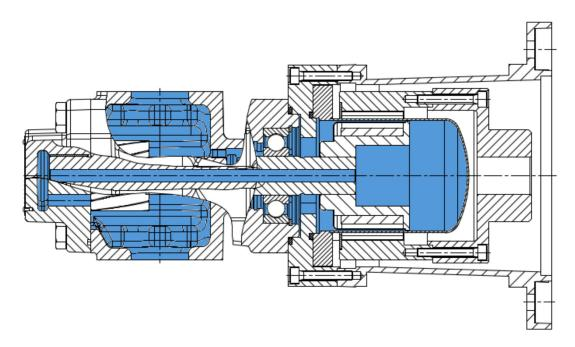
Versions with magnetic coupling are used when absolute leak-proofness is required on the shaft seal or when being operated with supply pressure on the suction side. The magnetic coupling is leak-proof within the permissible technical limits.
