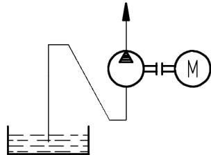
In case of longer suction lines that can run empty during the standstill, it is useful to insert a foot valve or a non-return valve. These must have been designed for use in suction lines and should offer as low a flow resistance as possible.
