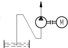
In case of longer suction lines that can run empty during the standstill, it is useful to insert a foot valve or a non-return valve. These must have been designed for use in suction lines and should offer as low a flow resistance as possible.
