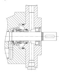
Mechanical seal with fluid buffer KF 32-80: Connection borehole G 1/4 (for fluid buffer)
