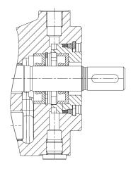
Double rotary shaft seal Connection borehole G 1/8
