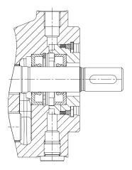
Double rotary shaft seal (for vacuum operation) Connection borehole G 1/8 (for fluid buffer) Special number: 74
