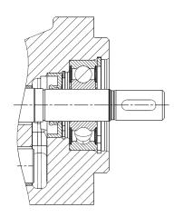
Rotary shaft seal with roller bearings
